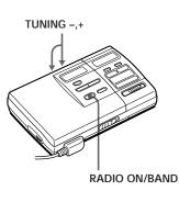
1 Press RADIO ON/BAND to turn on the radio. Then press RADIO ON/BAND to select AM, FM1\* or FM2\*.
